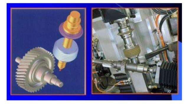
Fig, N°3 - Combination of worm wheel for high speed roughing and form wheel for high precision finishing.
