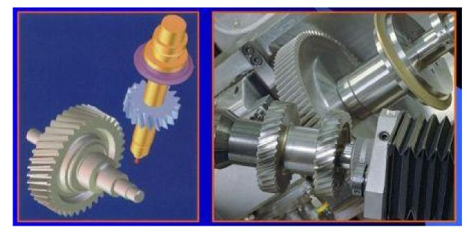
Fig.N°5 - Combination of a form wheel and a honing tool (external honing) for high precision grinding and profile finishing with lapping
