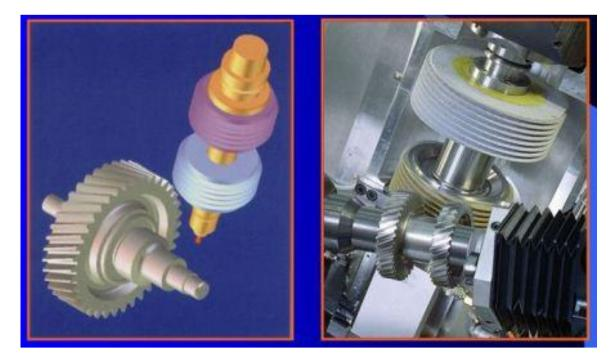
**Fig. N°4 -** Combination of two different types of worm wheels with two different grains for high-speed roughing and finishing or for grinding two different gears
